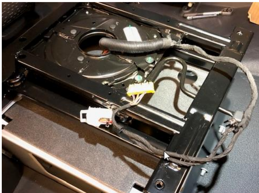
Passenger swivel seat base with seat harness unsecured (yellow and white connector).
